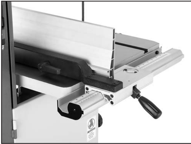
Figure 19. Correctly installed fence.
